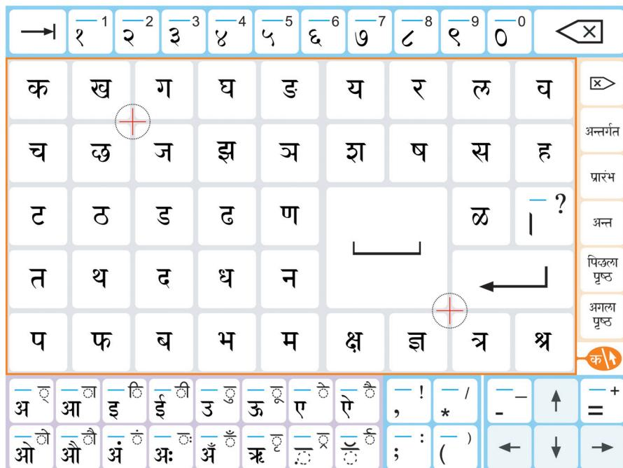
HFI collaborated with HP Labs to refine the design of the Gesture Keyboard, a text input device for non-English computer users. Based on the success of this design, HP is rolling out new versions of this keyboard for different languages at the rate of one per month.
